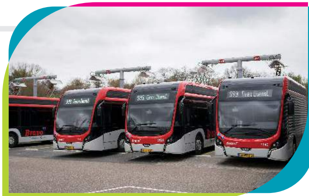
The buses during the charging and pre-heating of the battery
