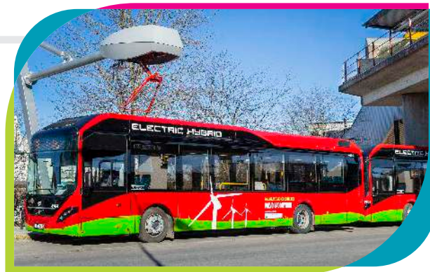
Charging Volvo Electric hybrid bus at the end station of route 73, at Ropsten in Stockholm
