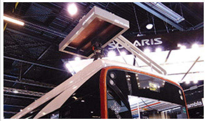
The overhead fast-charging system.
