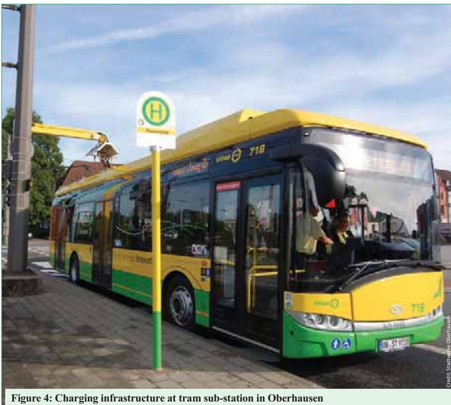
Figure 4: Charging infrastructure at tram sub-station in Oberhausen
