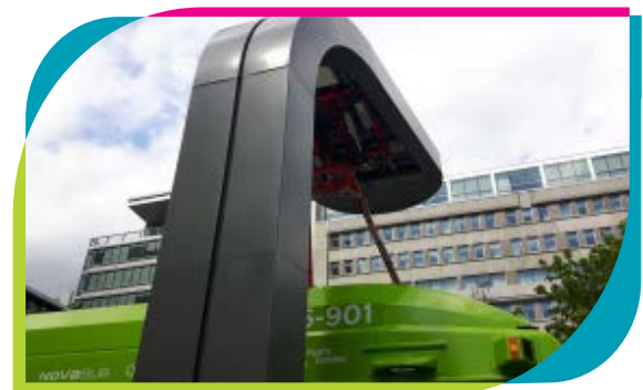
STM Pantograph charging station in Montreal Source: CBC
